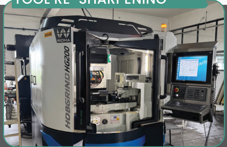
Hob Grind HG200, Broach Re-sharpening
